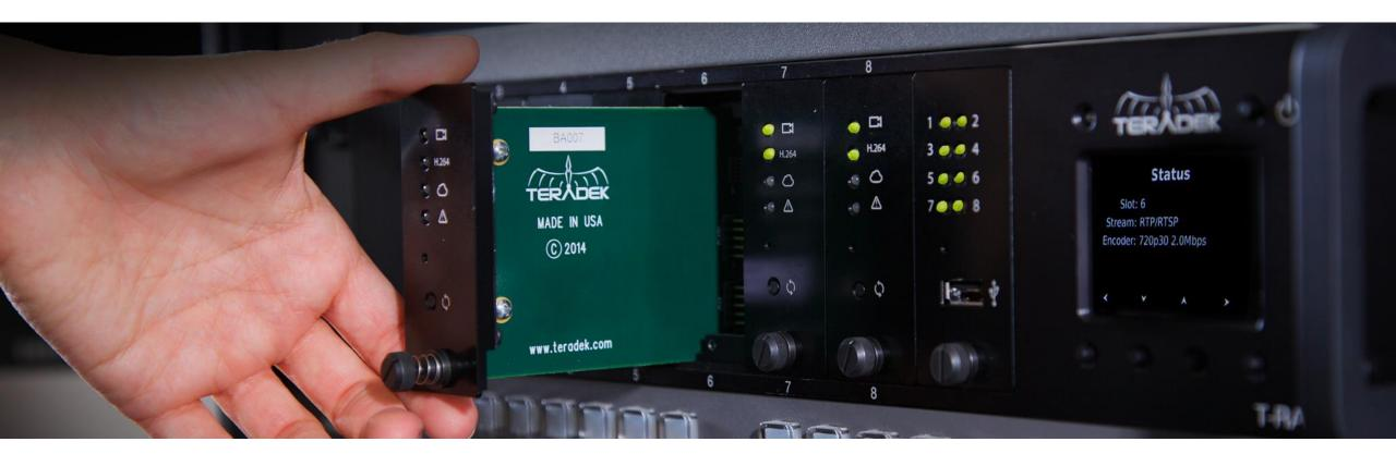
T-RAX is a high-density enterprise-grade H.264 platform that encodes, decodes, and streams video at broadcast quality
