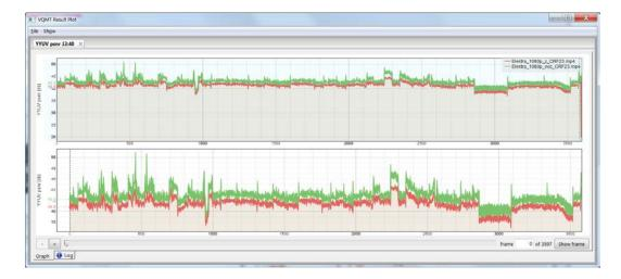
We used the Moscow State University Video Quality Measurement Tool (above) to identify any regions in the clip where quality might diverge. This compares the PSNR values of the processed (reddish) and unprocessed (green) clips. We checked all frames with significantly downward spikes, like those just before the 1000 frame marker on the left. You'll see such an analysis for each video we tested.
