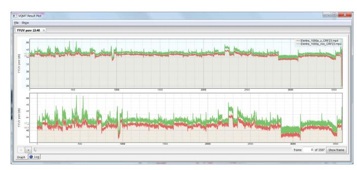
**Note drop off at end:** On several test clips, we noticed a quality drop at the very end resulting from a re-ordering of the last few frames. This is the sharp downward stroke of the red trace at the very right on top (clearer on the following page). We reported this in the first draft of this report. ZPEG sent a fix that we evaluate on the following page.
